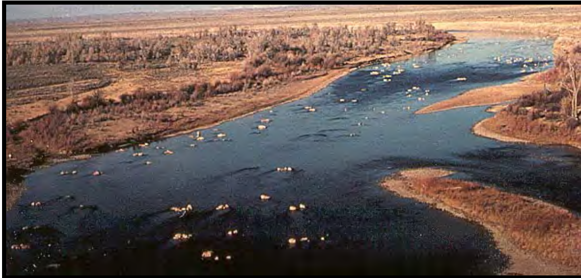
Figure 22-3. Granite boulders were added to the Green River downstream from Fontenelle Reservoir to increase shelter for trout.
