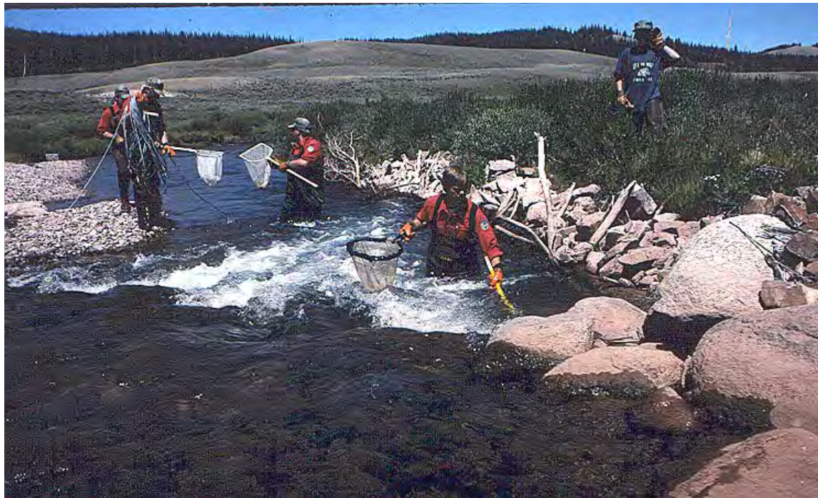
Figure 3. Fish population response to stream habitat improvement was regularly monitored with electrofishing gear at many WGF projects. This scene is at a diagonal rock weir on South Cottonwood Creek.
