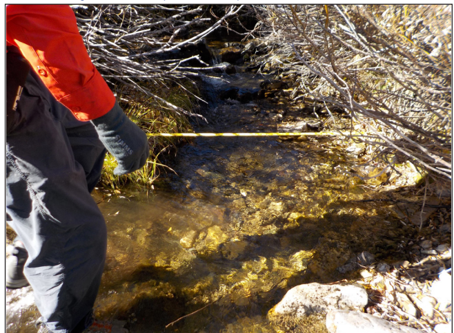
Figure 129. Flow measurement transect on Klondike Creek.
