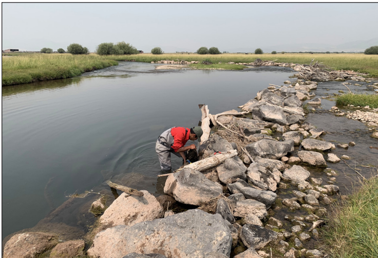
Figure 64. Deploying temperature loggers on the Salt River.
