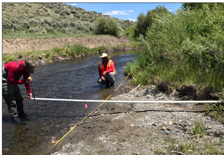
Figure 57. Measuring bankfull elevation, a key element of the Stream Quantification Tool.
