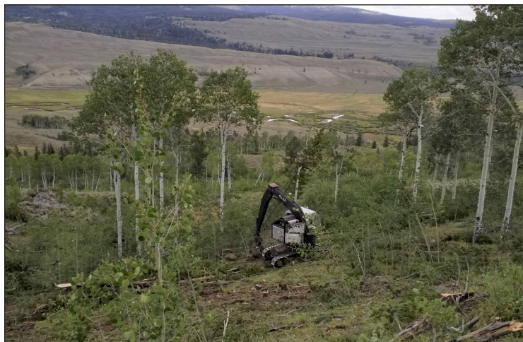
Figure 75. A Timbco feller buncher stacking felled material.
