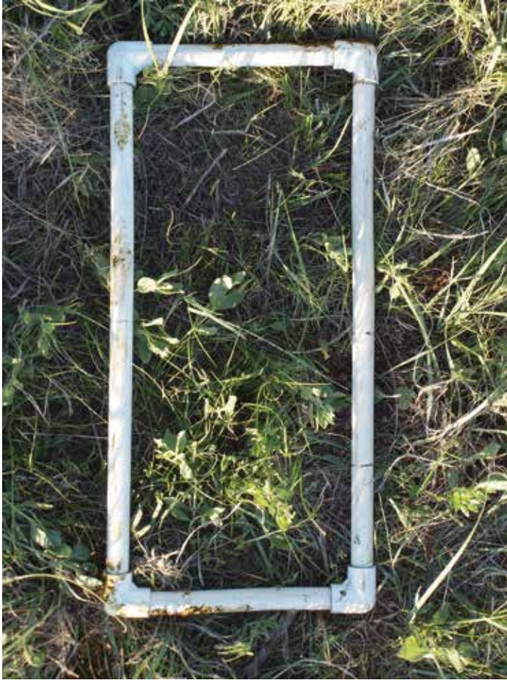
Figure A-3. A simple way to make a Daubenmire frame for estimating cover is to use PVC pipe cut to the dimensions of 20 x 50 cm.
