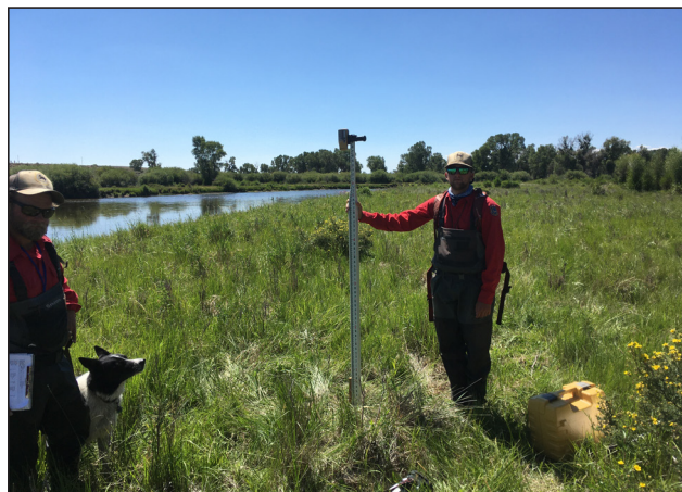
Figure 129. Using surveying equipment to establish a benchmark at the New Fork Gas Wells.
