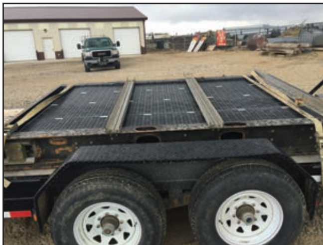
Figure 7. Vertical screen supports (metal bars in middle) after installation.
