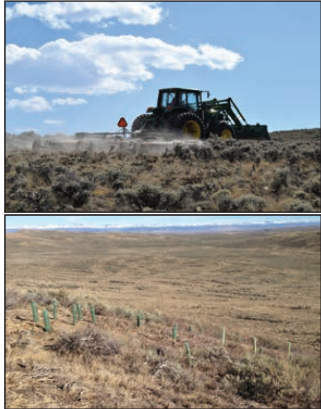
Figure 152. Mosaic big sagebrush thinning treatment with four wheel drive tractor and large brush mower.
