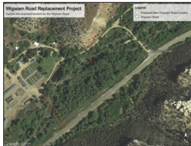
Figure 63. Aerial imagery showing the current and proposed location (in red) of the Wigwam Road and bridge crossing on Tensleep Creek.
