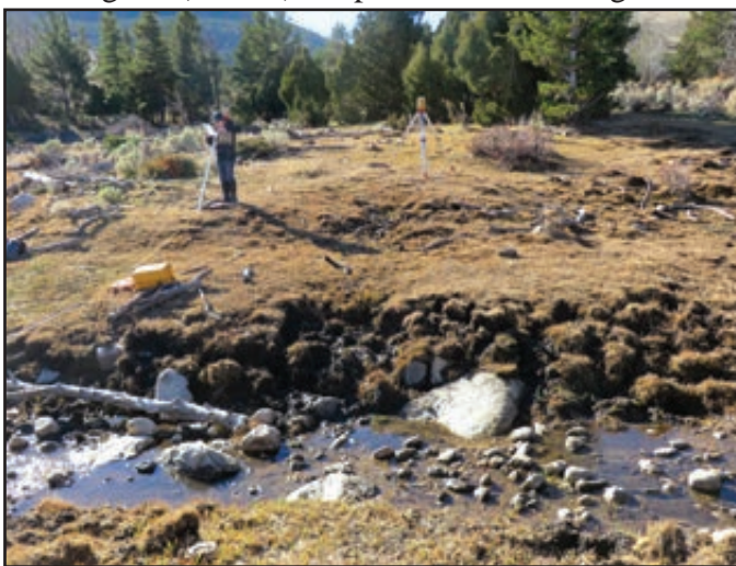
Figure 111. Setting up channel cross section transects at BDA locations.
