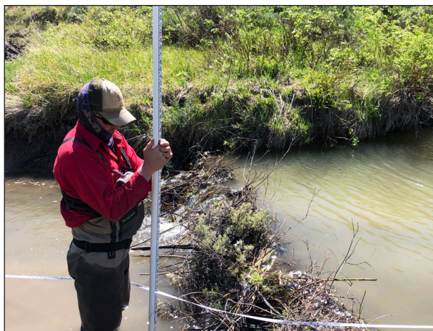
Figure 59. Luke Schultz surveys stream bed elevations at the Muddy Creek BDA control reach.
