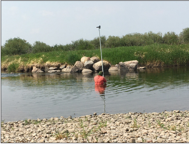
Figure 119. Collecting data on the Green River to measure the flow partitioning at a side channel.
