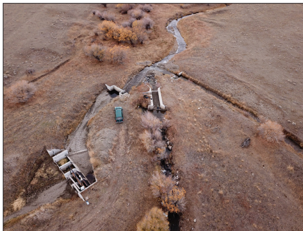
Figure 27. Main point of diversion on Timber Creek and the fish screen structure.
